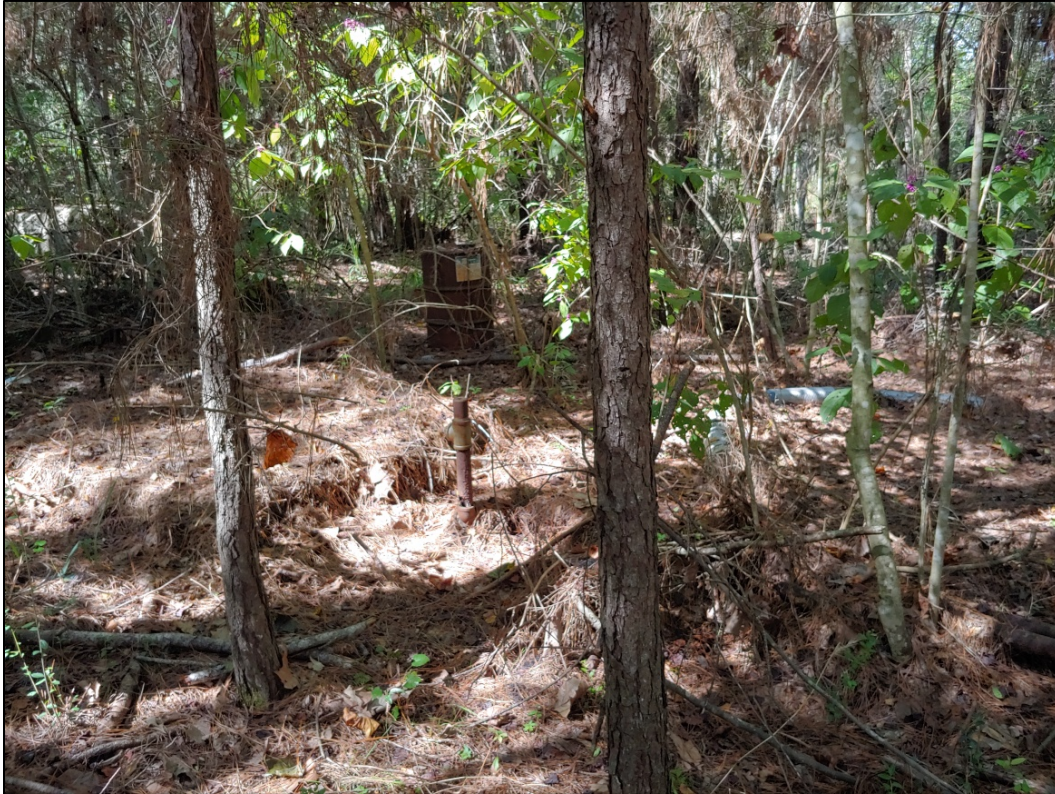
17. 55-gallon drum and piping associated with abandoned natural gas well.
